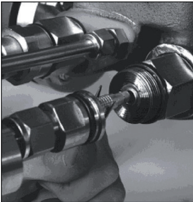
Figure 10: Disconnecting Lemo™ Connector
